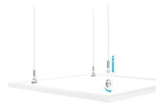
Standard ProSound ceiling rafts should have 4 spiral anchors that should be inserted in to the back of the ceiling raft 1 in each corner. All ProSound ceiling rafts will be supplied with the correct number of fixings for its size.
